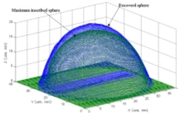
Fig. 6. The recovered sphere and the maximum inscribed sphere in the same coordinate.
