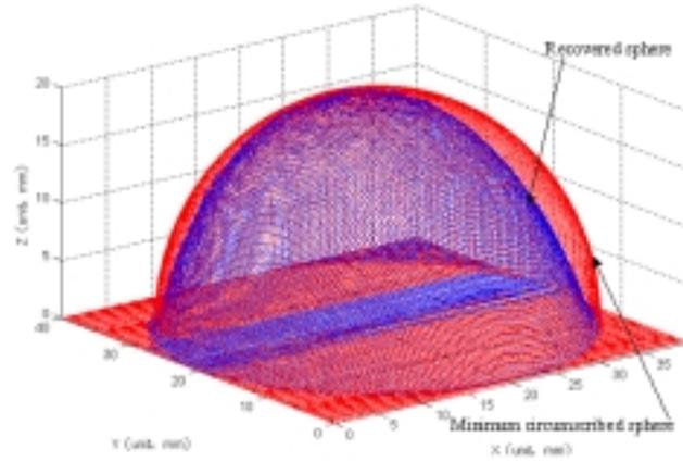
Fig. 5. The recovered sphere and the minimum circumscribed sphere in the same coordinate.
