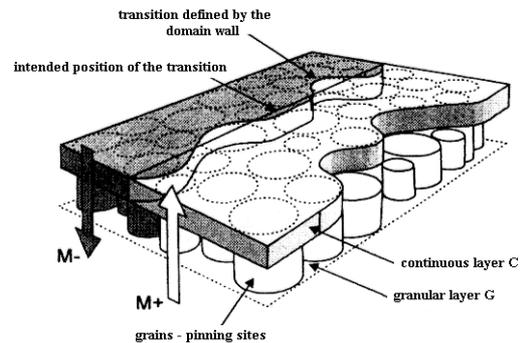
Fig.1 – The principle representation of a CGC medium. The location of the domain wall (of the transition) in the C layer is imposed by the orientation of the grains magnetization in the G layer [9].
