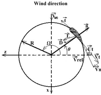
Fig. 1 – Two-dimensional rotor configuration.
