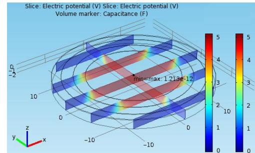
Fig. 12 – The electric potential and the capacitance of the cylindrical dermal drug delivery system.
