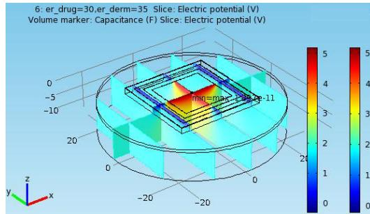
Fig. 11 – The electric potential and the capacitance of the parallelepipedical dermal drug delivery system.
