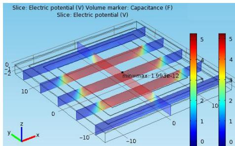
Fig. 7 – The electric potential and the capacitance of the parallelepipedical backing with build-in capacitor and empty patch.
