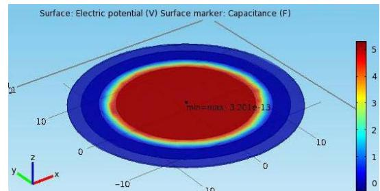
Fig. 5 – The electric potential and the capacitance of cylindrical capacitor.
