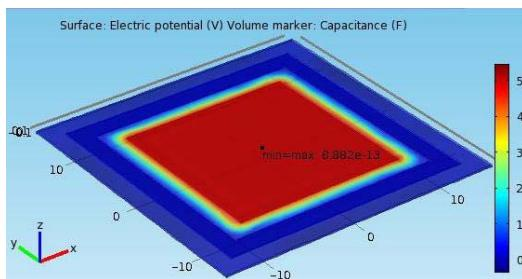
Fig. 4 – The electric potential and the capacitance of parallelepipedical capacitor.
