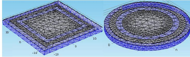
Fig. 6 – The representation of the mesh for the backing with built-in capacitor and drug-containing adhesive.
