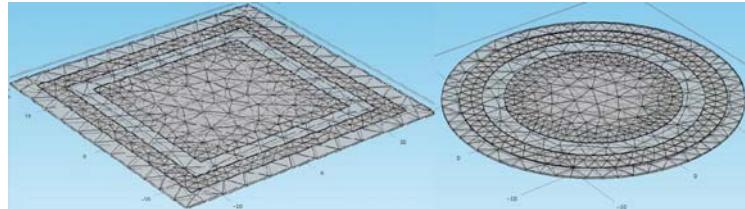
Fig. 3 – The representation of the mesh for the coplanar capacitors.
