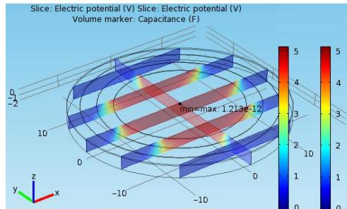
Fig. 8 – The electric potential and the capacitance of the cylindrical backing with build-in capacitor and empty patch.
