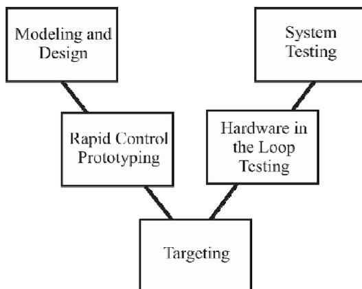
Fig. 1 – “V-Model” diagram for a development cycle based on rapid control prototyping.
