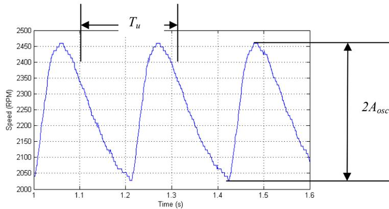
Fig. 7 – Controlled oscillation of the brushless direct current motor obtained using the relay feedback method.
