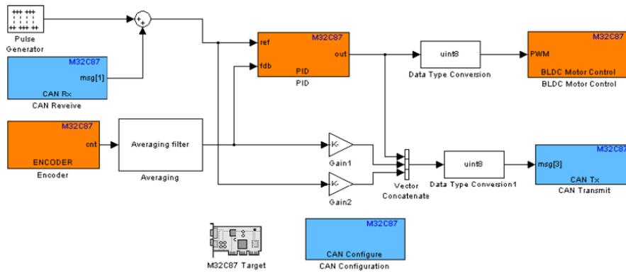
Fig. 10 – Simulink block diagram for closed loop control of brushless direct current motor.
