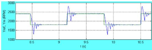
Fig. 8 – Closed loop step response using the PID controller determined with the Ziegler-Nichols tuning method.
