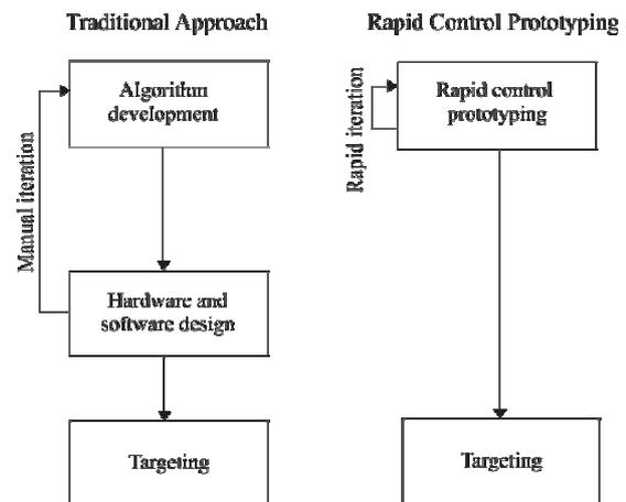
Fig. 2 – Comparison between the traditional and the rapid prototyping approach.
