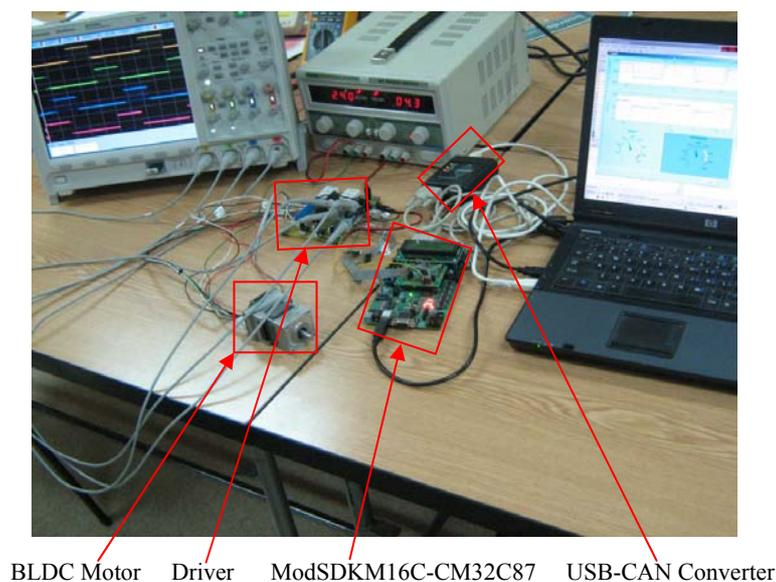
BLDC Motor Driver ModSDKM16C-CM32C87 USB-CAN Converter
