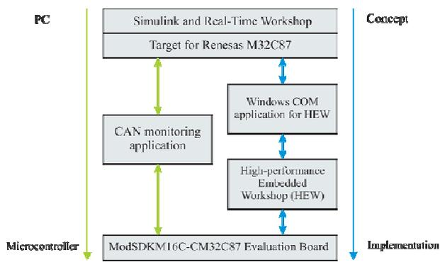
Fig. 3 – Block diagram for the information and data flows for the *Target for Renesas M32C87* rapid control prototyping toolbox.
