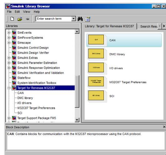
Fig. 4 – *Target for Renesas M32C87* Matlab rapid control prototyping toolbox.
