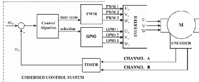
Fig. 5 – Block diagram for closed loop control of BLDC motor.
