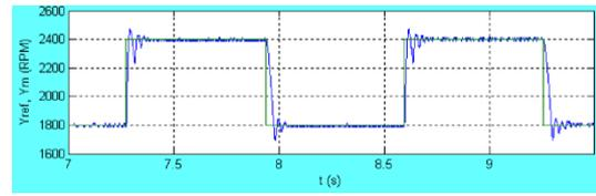
Fig. 9 – Closed loop step response using the PID controller tuned with a specified phase margin.
