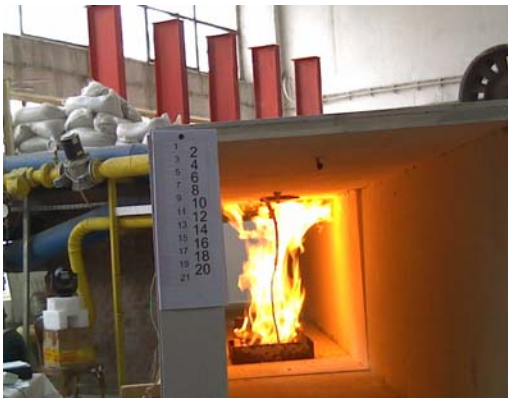
Fig. 8 – View of the reduced scale tunnel during the experimental test.
