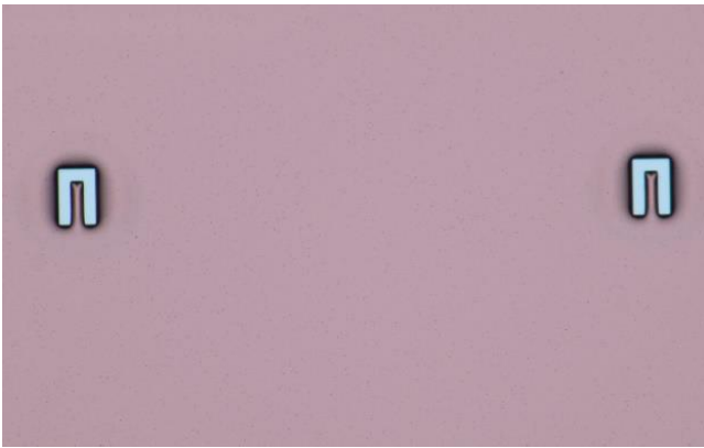
Fig. 4 – Piezoresistive formation by ion injection.
